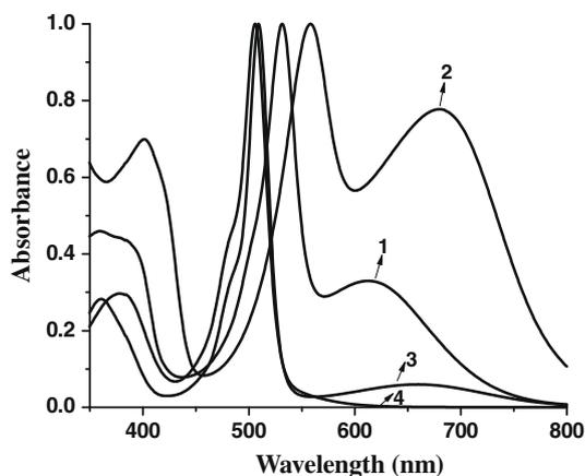
Fig. 4. Absorption spectra of BODIPY–ferrocene conjugates **1–4** recorded in toluene. The concentration used was  $5 \times 10^{-5}$  M.
