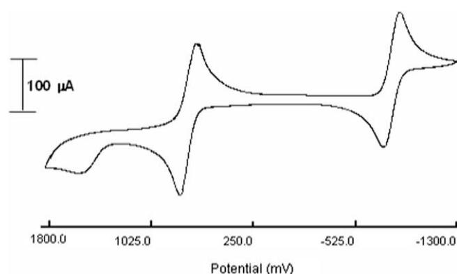
Fig. 5. Cyclic voltammogram of compound **3** in dichloromethane containing 0.1 M TBAP as supporting electrolyte recorded at  $50 \text{ mV s}^{-1}$  scan speed.
