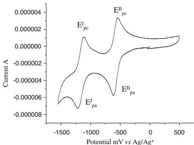
**Figure 3.** Cyclic voltammogram of compound **11** in 0.1 M Et<sub>4</sub>NBF<sub>4</sub>/acetonitrile obtained in Pt electrode, scan rate 100 mV/s. The cathodic ( $E_{pc}^I$ ,  $E_{pc}^{II}$ ) and anodic ( $E_{pa}^I$ ,  $E_{pa}^{II}$ ) peak potentials are indicated in the figure.
