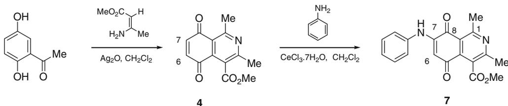
Scheme 1. Preparation of 7-anilinoisoquinolinequinone 7.
