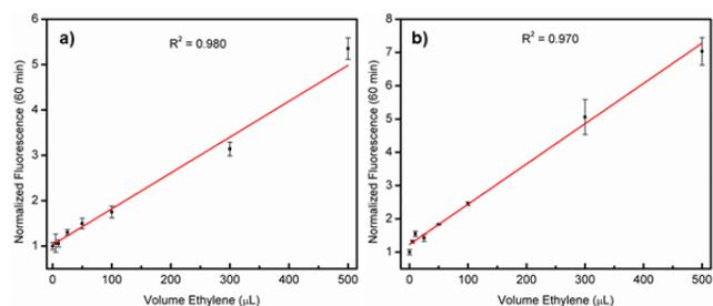
**Figure 3.** BEP-4 and BEP-5 in toluene show turn-on response to ethylene gas injected via gas tight syringe. Turn-on fluorescence response of 2  $\mu$ M (a) BEP-4 or (b) BEP-5.  $\lambda_{ex} = 475$  nm,  $\lambda_{em} = 513$  nm (BEP-4) and 514 nm (BEP-5). Endpoints represent normalized fluorescence 60 min after the addition of ethylene. Error bars denote SD.
