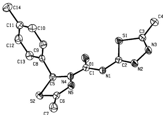
Figure 3. Molecular structure and numbering of **2a**. Thermal ellipsoids are drawn at the 40% probability level. Hydrogen atoms have been omitted for clarity. Selected bond lengths [pm] and angles [°]: N2–N3 139.5(3), N1–C2 138.0(3), C1–N1 137.9(3), C1–O1 122.6(3), C1–N4 135.9(3), N4–N5 147.5(3), C1–N1–C2 121.1(2); O1–C1–N4 121.4(2), O1–C1–N1 123.1(2), N4–C1–N1 115.5(2).
