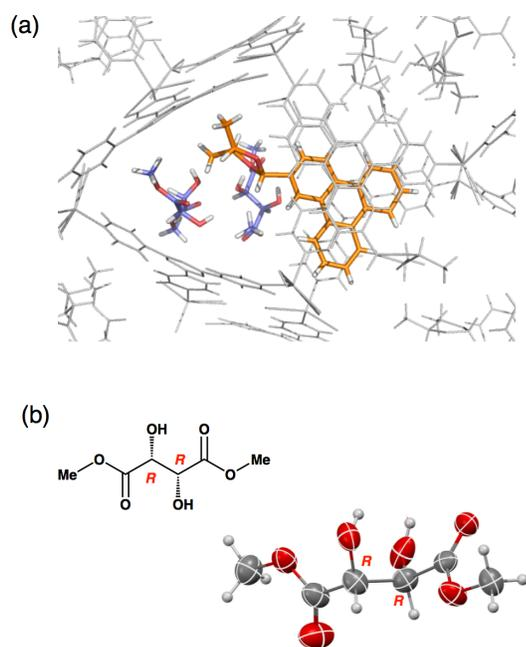
**Figure 2.** (a) X-ray structure of (*S,S*)-**1**•(*2R,3R*)-**3**. The analyte (*2R,3R*)-**3** and the chiral reference, (*S,S*)-**1**, plugged in the host framework are highlighted in color. (b) ORTEP drawing of (*2R,3R*)-**3**. Thermal ellipsoids are shown at the 50% probability level. Its *R,R* configuration was confirmed by comparing the relative configuration to the chiral reference, (*S,S*)-**1**.
