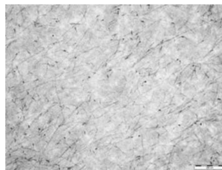
Fig. 4 TEM image of cross section of the poly(styrene–DVB) wafer created in the presence of gelator 1 (20 mM). Reactive staining agent: OsO 4 . Scale bar: 200 nm.
