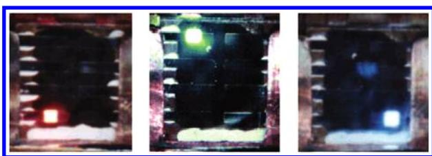
**Figure 6.** Electroluminescence from devices using polymers **9** (left), **7** (center), and **11** (right).
