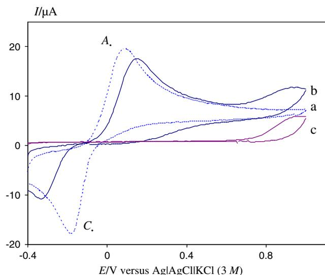
**Fig. 1** Cyclic voltammograms of 2 mM 2,3-dimethylhydroquinone (1) in the absence *a* and presence *b* of 2 mM 4-hydroxy-1-methyl-2(*I*H)-quinolone (3a); (*c*) cyclic voltammogram of 2 mM 3a at a glassy carbon electrode (1.8 mm diameter) in a mixture of water-acetonitrile (80:20) containing 0.20 M phosphate ( $\text{KH}_2\text{PO}_4/\text{K}_2\text{HPO}_4$ ) solution of pH 7.0. Scan rate:  $100 \text{ mV s}^{-1}$ ;  $t = 25 \pm 1 \text{ }^\circ\text{C}$
