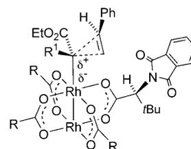
Scheme 1. Carbene-transfer step during styrene cyclopropanation with a carbene generated from a diazoester mediated by [Rh<sub>2</sub>{(*S*)-pttl}<sub>4</sub>].
