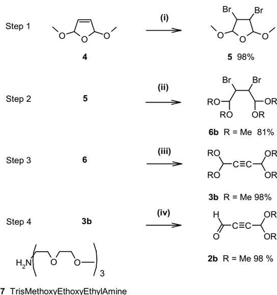
**Scheme 3.** Synthesis of acetal **3a** from dimethoxydihydrofuran. Reactions conditions: (i) Br<sub>2</sub>, CH<sub>2</sub>Cl<sub>2</sub> (98%); (ii) MeOH, H<sub>2</sub>SO<sub>4</sub> (81%); (iii) THF, KOH, TMEEA (98%); (iv) HCO<sub>2</sub>H/CH<sub>2</sub>Cl<sub>2</sub> (98%).
