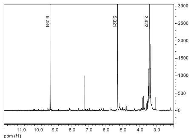
**Figure 3.** NMR spectrum of the crude monoacetal **2b** showing the main impurities.
