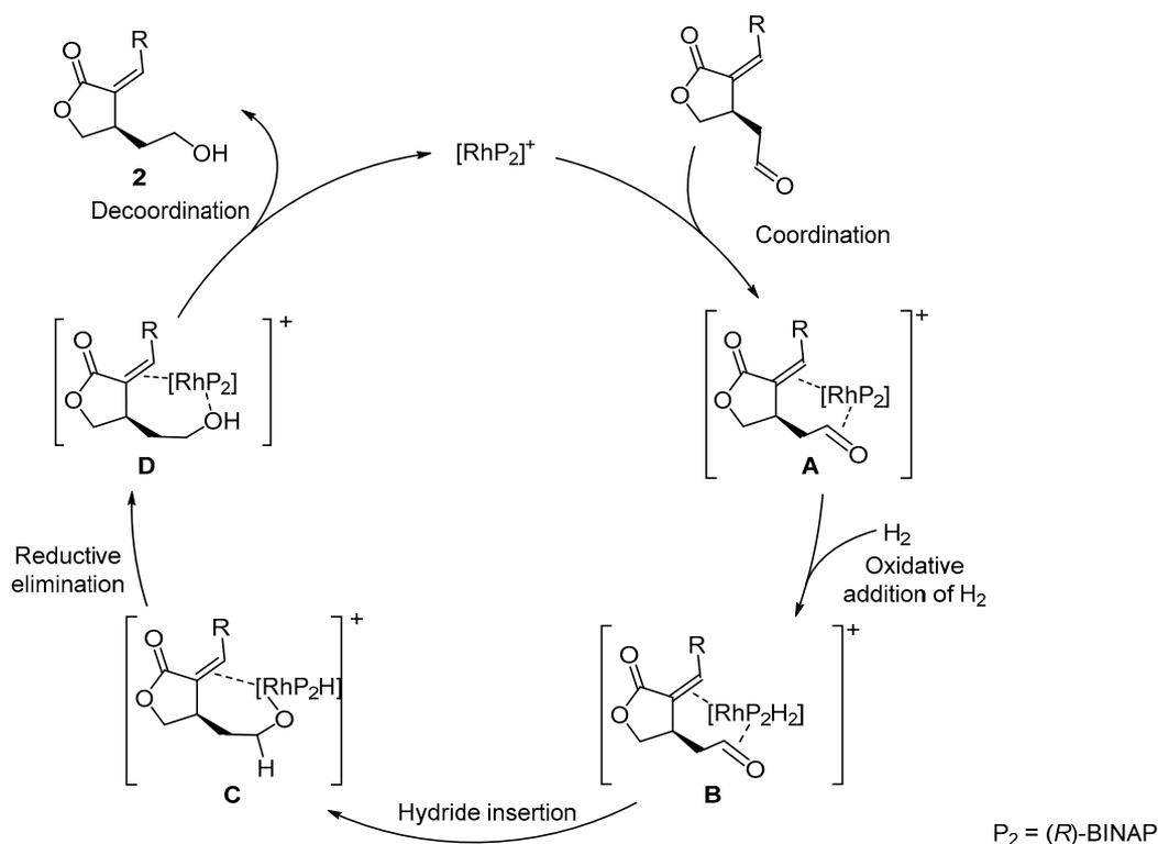
Rh-(*R*)-BINAP complex, the chelated complex **A** undergoes oxidative addition to give the dihydrido complex **B**. Hydride insertion furnishes the Rh-alcoholate **C**, which undergoes reductive elimination to generate the alcohol complex **D**. After decooordination of product **2**, the cationic Rh-(*R*)-BINAP complex is ready for a new catalytic cycle.
