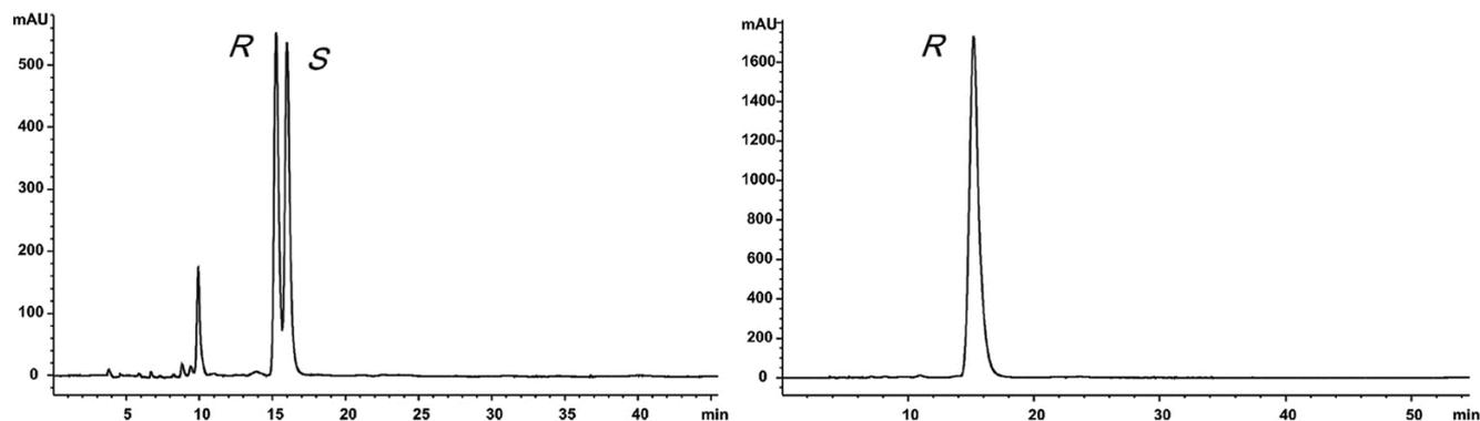
**Figure 3.** Analytical chiral HPLC chromatograms of (*rac*)-**5b** (left) and (*R*)-**5b** (right) (HPLC: *n*-hexane–2-PrOH 95:5, 0.8 ml/min,  $\lambda_{\text{exc}}$  266 nm, retention times:  $t_R$  15.2 min (major),  $t_S$  16.0 min (minor)).
