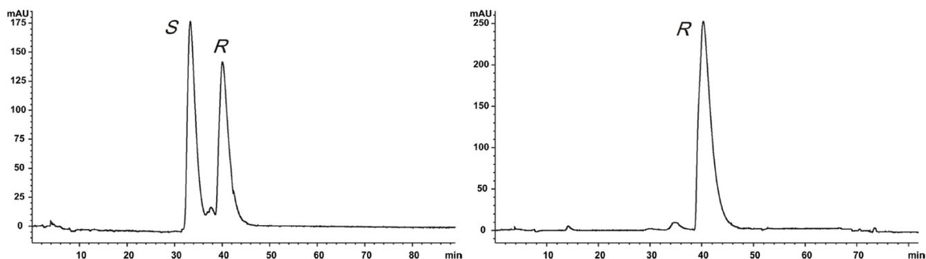
**Figure 1.** Analytical chiral HPLC chromatograms of (*rac*)-**3** (left) and (*R*)-**3** (right) (HPLC: *n*-hexane–2-PrOH, 95:5, 0.8 ml/min,  $\lambda_{\text{exc}}$  254 nm, retention times:  $t_S$  33.3 min (minor),  $t_R$  40.2 min (major)).
