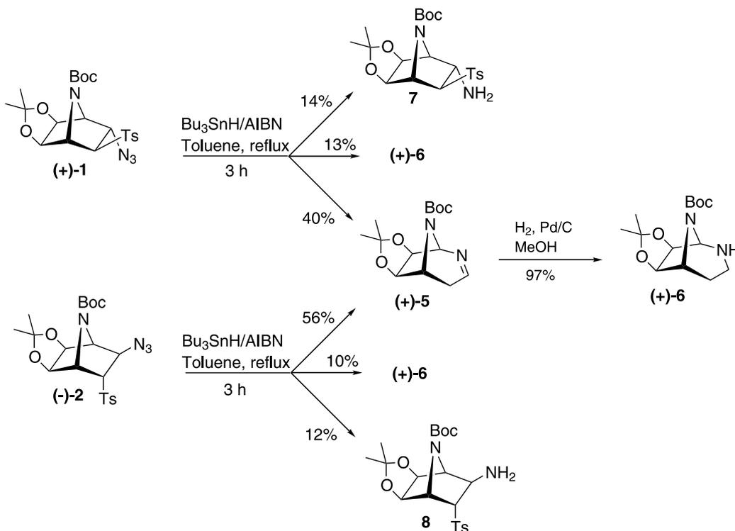
**Scheme 2.** Ring expansion in the reductive desulfonylation of β-azido sulfones (+)-1 and (-)-2.
