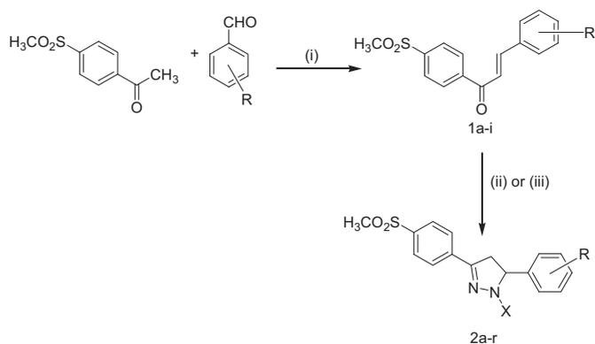
Scheme 1. Reagent and conditions: (i) Ba(OH)<sub>2</sub>·8H<sub>2</sub>O, EtOH 96%, 25–30 °C, 8 h; (ii) NH<sub>2</sub>NH<sub>2</sub>, CH<sub>3</sub>COOH, EtOH dry, 78 °C, 24 h; (iii) NH<sub>2</sub>NHCSNH<sub>2</sub>, NaOH, EtOH dry, 78 °C, 24 h (for assignment of a–r see Table 1).
