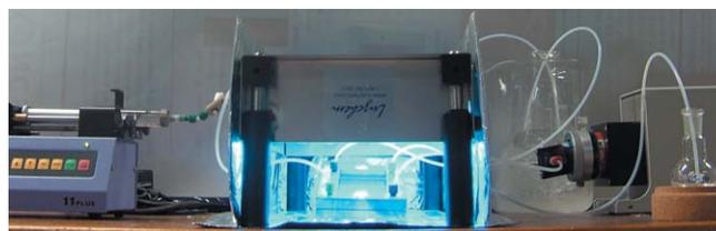
**Figure 1** Microreactor (dwell device, mikroglas) under a UV exposure panel (Luzchem)
