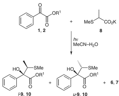
**Scheme 2** Addition of potassium 2-(methylsulfanyl)propionate **8** to **1/2****Table 2** Product Compositions and Experimental Details for Photoadditions of **1/2** with **8**
