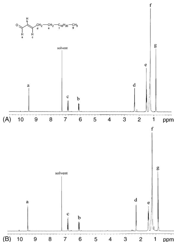
Fig. 5. NMR analysis of 2-hexadecenal. Semi-synthetic 2-hexadecenal (A) and the putative 2-hexadecenal product from MPO-derived RCS targeting of SPC (B) were prepared and subjected to proton NMR as described in Section 2. Peak assignments are shown in inset in Fig. 4A.
