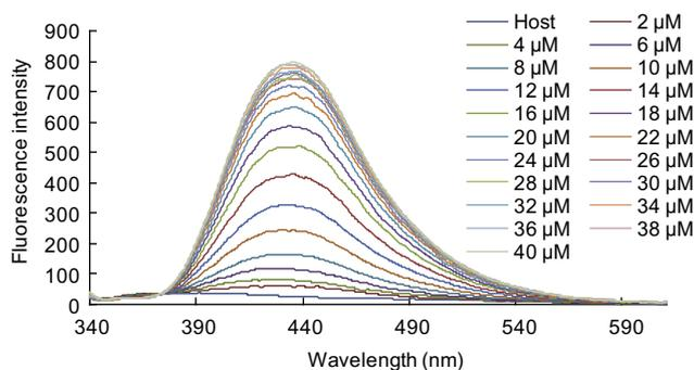
**Figure 3.** Fluorescence spectra changes of receptor **5** ( $10 \mu\text{M}$ ) upon adding  $\text{Zn}(\text{NO}_3)_2$  in  $\text{CH}_3\text{CN}/\text{DMSO}=99:1$  ( $\lambda_{\text{ex}}=323 \text{ nm}$ ).
