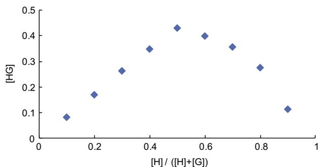
**Figure 5.** Job's plot between receptor **5** and  $\text{Zn}^{2+}$ . The  $[\text{HG}]$  concentration was calculated by the equation  $[\text{HG}] = \Delta I/I_0 \times [H]$ .
