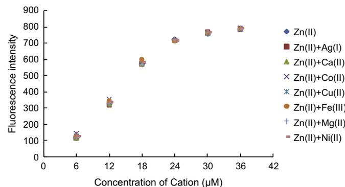
Figure 8. Estimating  $\text{Zn}^{2+}$  ions with receptor **5** ( $10\ \mu\text{M}$ ) in the presence of equimolar metal ions in  $\text{CH}_3\text{CN}/\text{DMSO}$  (99:1, v/v) at 432 nm.
