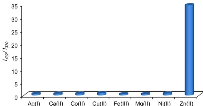
**Figure 2.** Ratiometric fluorescence ( $I_{432}/I_{370}$ ) response of receptor **5** ( $10 \mu\text{M}$ ) upon adding a particular metal salt ( $40 \mu\text{M}$ ) in  $\text{CH}_3\text{CN}/\text{DMSO}=99:1$ .
