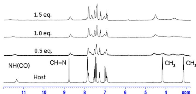
**Figure 6.** Family of  $^1\text{H}$  NMR spectra of receptor **5** upon adding  $\text{Zn}^{2+}$  ions in  $\text{DMSO}-d_6$ .
