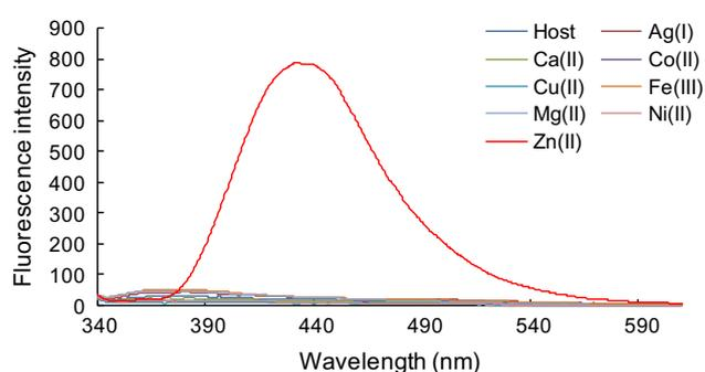
Figure 1. Changes in fluorescence intensity of receptor **5** ( $10\ \mu\text{M}$ ) upon adding particular metal ions ( $40\ \mu\text{M}$ ) in  $\text{CH}_3\text{CN}/\text{DMSO}=99:1$  ( $\lambda_{\text{ex}}=323$  nm).
