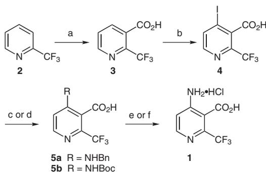
**Scheme 3** Synthesis of 4-amino-2-(trifluoromethyl)nicotinic acid. *Reagents and conditions:* (a) LTMP, –70 °C, then CO<sub>2</sub> (g) or dry ice, 77%; (b) LTMP, –70 °C; then I<sub>2</sub>; (c) BnNH<sub>2</sub>, 120 °C, then Ac<sub>2</sub>O, Et<sub>3</sub>N; (d) BocNH<sub>2</sub>, Pd<sub>2</sub>(dba)<sub>3</sub>, Xantphos, Cs<sub>2</sub>CO<sub>3</sub>, *tert*-amyl alcohol, 84%; (e) H<sub>2</sub> (100 psi), Pd(OH)<sub>2</sub>/C, MeOH, AcOH, 50 °C, 73%; (f) HCl (g), MeOH, 100%.
