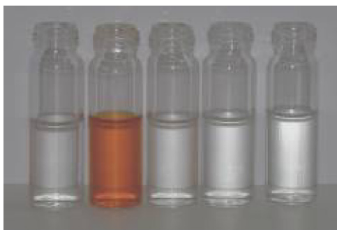
Figure 3. Colour changes of receptor ( R ) 1 in \text{CH}_3\text{CN} ( 5.0 \times 10^{-5} M) before and after the addition of 2 equiv of representative anions (from left to right: R , R + \text{F}^- , R + \text{Cl}^- , R + \text{Br}^- , R + \text{I}^- ).
