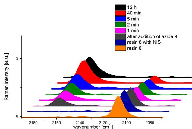
**Figure 2.** Real time monitoring of the on-bead transformation of alkyne **8** to nitrile **6** via Raman spectroscopy of the reaction mixture.
