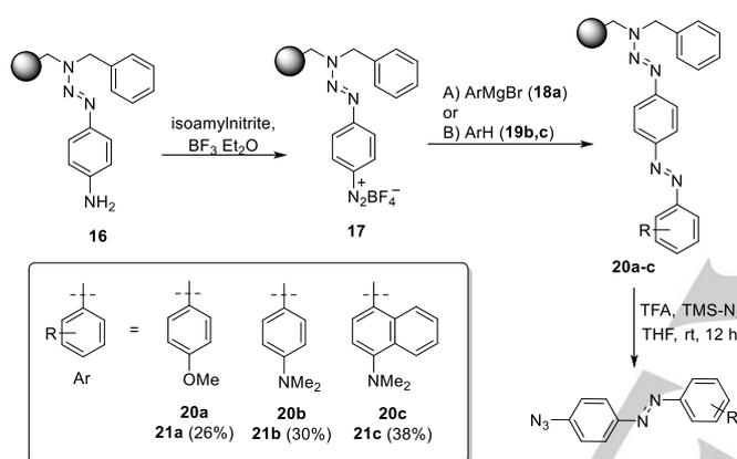
**Scheme 6.** Synthesis of azo-containing compounds **21a-c** on a triazene-linker.
