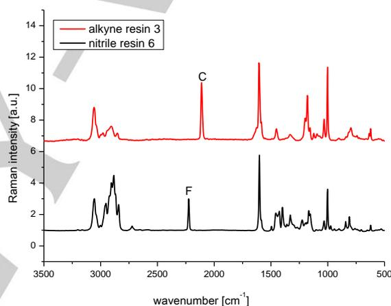
**Figure 1.** Monitoring of the successful immobilization of functionalized building blocks (see Table 1 for the assignment of bands C and F).
