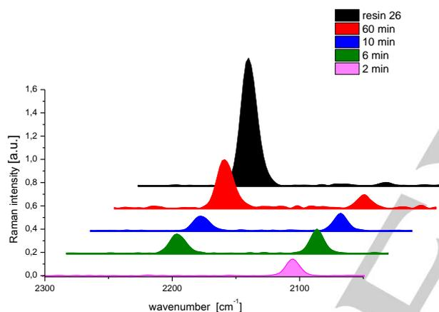
**Figure 3.** Real-time reaction monitoring of the Sonogashira reaction of solid-supported aryl iodide with ethynylbenzene (**25a**) to **26**.
