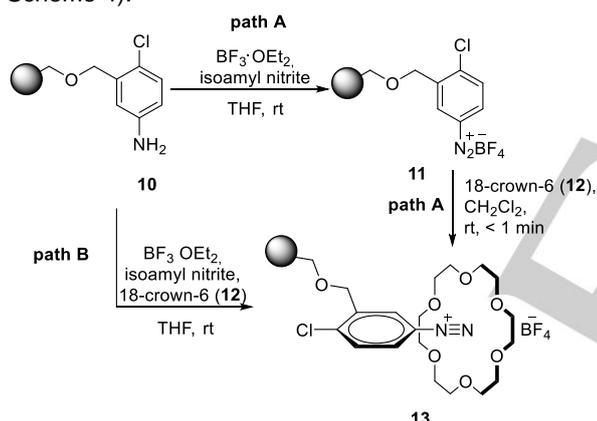
**Scheme 4:** Exemplarily chosen diazotization-masking protocol; path A: reaction of aniline **10** to the corresponding diazonium tetrafluoroborate **11** and subsequent masking with 18-crown-6 (**12**); path B: one-pot procedure to the target resin **13**.
