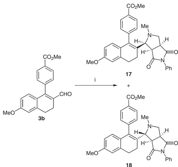
**Scheme 4** Reagents and conditions: *i.* *N*-phenylmaleimide, sarcosine, xylene, reflux, 61%.
