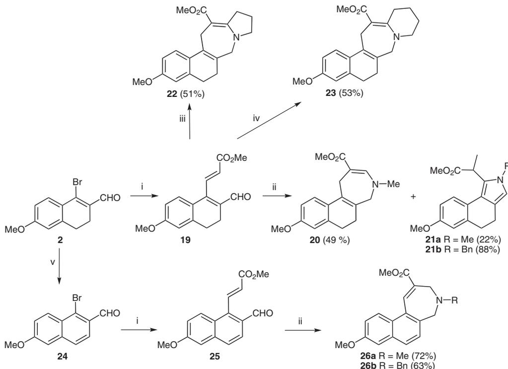
**Scheme 5** Reagents and conditions: *i.*  $\text{CH}_2=\text{CHCO}_2\text{Me}$ ,  $\text{Pd}(\text{OAc})_2$ ,  $\text{P}(o\text{-tolyl})_3$ ,  $\text{Et}_3\text{N}$ , DMA, 120 °C, 3 h (82%); *ii.* sarcosine (R = Me) or *N*-benzylglycine (R = Bn), xylene, reflux; *iii.* **12**, xylene, reflux; *iv.* **10**, xylene, reflux; *v.* DDQ,  $\text{CHCl}_3$ , 60 °C, 48 h (65%).
