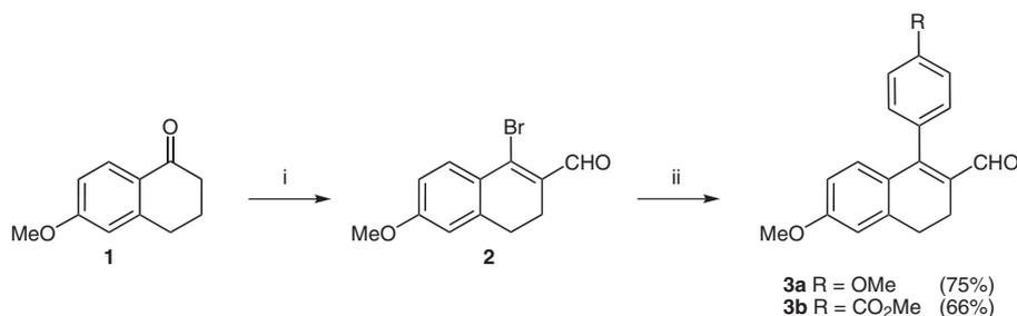
**Scheme 1** Reagents and conditions: *i*. DMF, PBr<sub>3</sub>; *ii*. ArB(OH)<sub>2</sub>, Pd(OAc)<sub>2</sub>, P(*o*-tolyl)<sub>3</sub>, Na<sub>2</sub>CO<sub>3</sub>.
