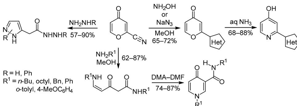
2-Cyano-4-pyrone obtained from comanic acid ethyl ester reacts with amines and hydrazines with the opening of the pyrone ring and substitution of the cyano group to form carbamoylated aminoenones (yields 62–87%) and pyrazolylacetic acid hydrazides. The reactions of 2-cyano-4-pyrone with hydroxylamine or sodium azide involve exclusively the cyano group, which makes it possible to obtain 2-heteroaryl-4-pyrones and 2-heteroaryl-4-hydroxypyridines.
