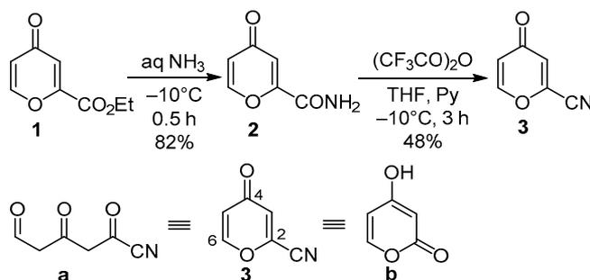
As starting material for the preparation of 2-cyano-4-pyrone (**3**), comanic acid ethyl ester (**1**) was used which was first converted to amide **2**.<sup>7</sup> It must be taken into account that the pyrone ring is easily opened by the action
