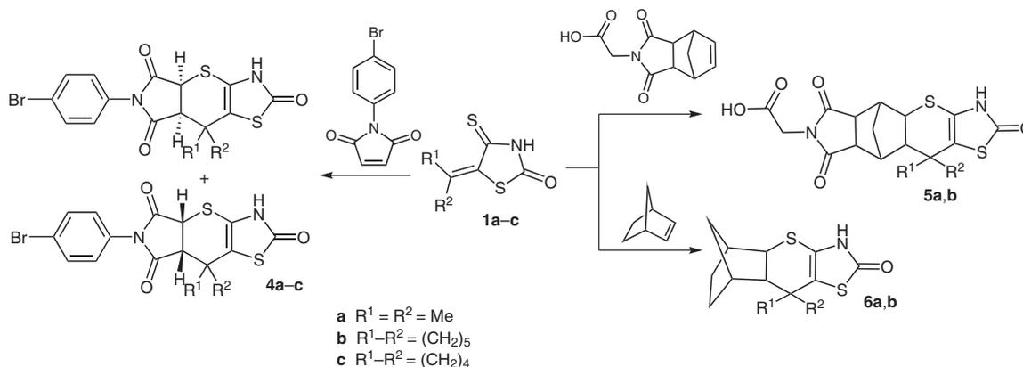
**Scheme 3** Synthesis of new thiopyrano[2,3-d][1,3]thiazol-2-one derivatives (**4–6**). *Reagents and conditions:* **1** (1.0 equiv), dienophile (1.2 equiv), hydroquinone, AcOH, reflux, 1 h.
