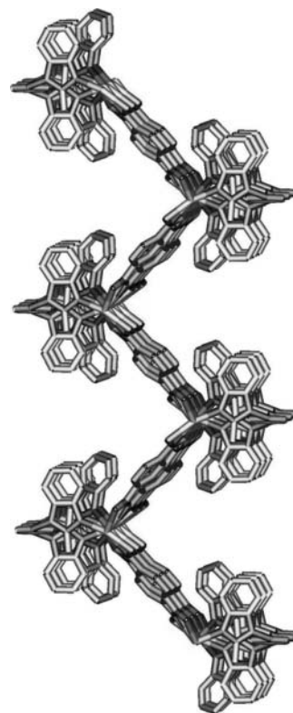
FIG. 2. The 1D \text{Cd}/p\text{-bdc}^{2-} zigzag chains are linked by bmb to generate a 2D puckered network.
