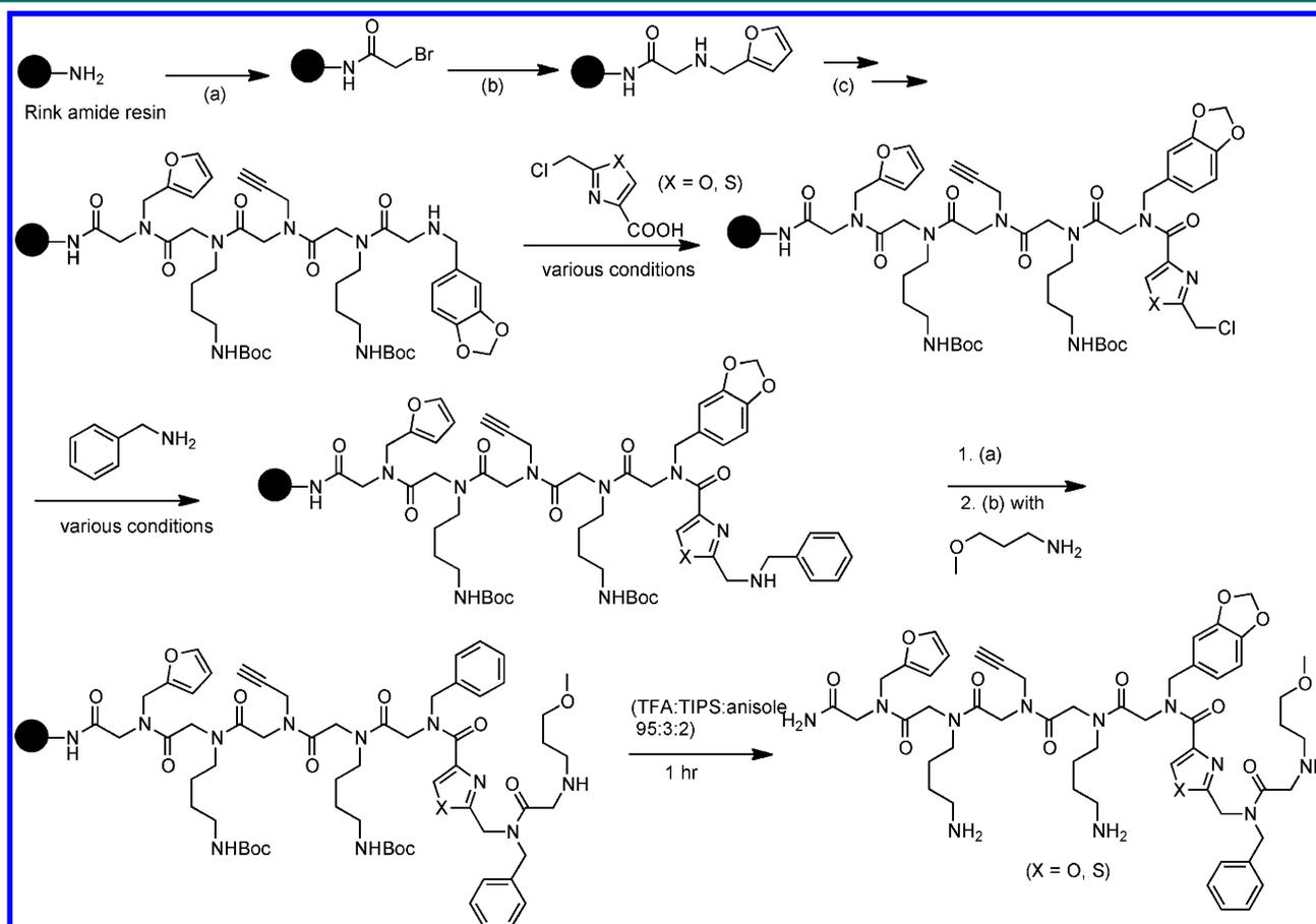
**Figure 2.** Incorporation of azole heterocycles to generate a backbone modified peptoid (a) BrCH<sub>2</sub>COOH (2 M in DMF), DIC (2 M in DMF), MW 15 s, 10% power (100 W) repeated twice. (b) Primary amine (2 M in DMF), MW 30 s, 10% power (100 W) repeated three times. (c) Steps (a) and (b) repeated four times with various amines. Different conditions for acylation with the heterocycle and subsequent displacement with the amine are described in Table 1.
