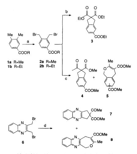
a) NBS, (PhCOO)<sub>2</sub>, CCl<sub>4</sub>, 2h, reflux. b) (EtOCO)<sub>2</sub>CH<sub>2</sub>, K<sub>2</sub>CO<sub>3</sub>, butanone, 18h, reflux. c) MeCOCH<sub>2</sub>COOMe, K<sub>2</sub>CO<sub>3</sub>, butanone, 20h, reflux. d) MeCOCH<sub>2</sub>COOMe, K<sub>2</sub>CO<sub>3</sub>, acetone, 6h, reflux.
