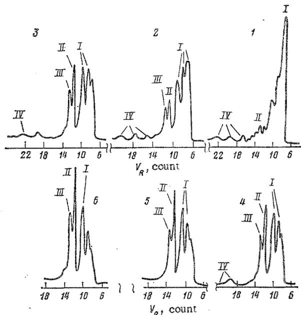
Fig. 1. Gel chromatograms of the products of the alcoholysis (or decomposition) of the oligomeric ether (II) ( $C_0$  48.1 g/liter) with ethanol ( $COC_2H_5OH$  1.856 mole/liter) in the presence of *p*-toluenesulfonic acid ( $C_{cat}$   $6.31 \cdot 10^{-3}$  mole/liter) at 95-110°C for (min): 1) 40, 2) 80, 3) 121, 4) 140, 5) 161, 6) 194; peaks: (I) oligomeric and dimeric alcoholysis products of the ether (II); (II) ether (VIa); (III) ether (VIIa); (IV) hydroxylated alcoholysis products of (V).
