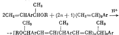
Hence, the acid-catalyzed reactions of the diol (I)-alkanol and diol (I)-carboxylic acid systems are analogous. Furthermore, both series of reactions result in the formation of the same divinylaromatic compounds and the products of their polyaddition by the formation of straight-chain unsaturated styrene dimers.
