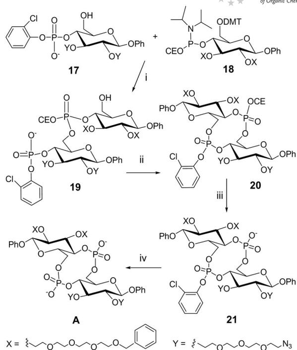
Scheme 7. Synthetic scheme for the preparation of cyclic dimer **A**: Reagents and conditions: (i) (a) DCI (0.25 M in  $\text{CH}_3\text{CN}$ ), room temp., 2 h; (b) *t*ButOOH (5.5 M in decane), room temp., 30 min; (c) on-column detritylation (74% for the three steps); (ii) DMAP, MSNT, Py, room temp., 12 h (75%); (iii) piperidine,  $70^\circ\text{C}$ , 12 h (quant.); (iv) satd. aq. LiOH/dioxane (5:1),  $50^\circ\text{C}$ , 12 h (96%).
