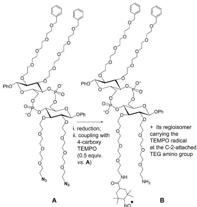
Figure 4. Conversion of azido-functionalized CyPLOS **A** into spin-labeled **B** – obtained as a mixture of regioisomers – through azide reduction followed by coupling with 4-carboxy TEMPO. Reagents and conditions: (i) (a)  $\text{Ph}_3\text{P}$ , THF, room temp., 12 h; (b)  $\text{H}_2\text{O}$ , room temp., 48 h (quant.); (ii) 4-carboxy-TEMPO, DIPEA, DCC, room temp., 12 h (67%).
