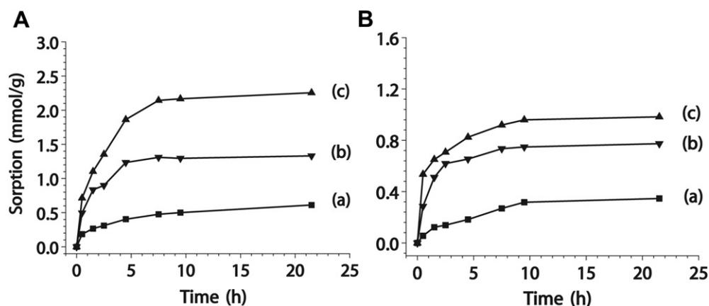
**Fig. 3.** The sorption of (A) Cd<sup>2+</sup> and (B) Pb<sup>2+</sup> as a function of the time for the PSt sub-micron spheres with the zeta potential: (a) -26.0 mV, (b) -51.3 mV, and (c) -70.7 mV.
