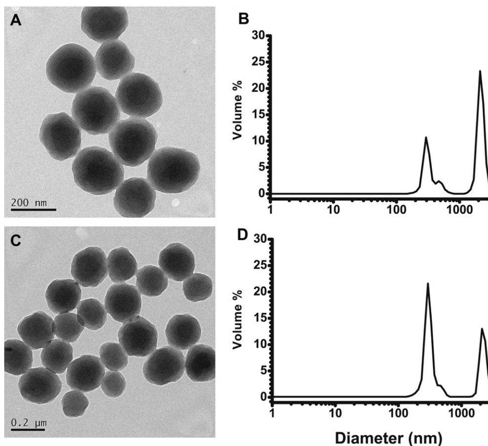
**Fig. 4.** TEM images and size distributions of PSt sub-micron sphere-Cd<sup>2+</sup> complex (A, B) and PSt sub-micron sphere-Pb<sup>2+</sup> complex (C, D). All the PSt sub-micron spheres before ion coordination have a zeta potential of -26.0 mV.
