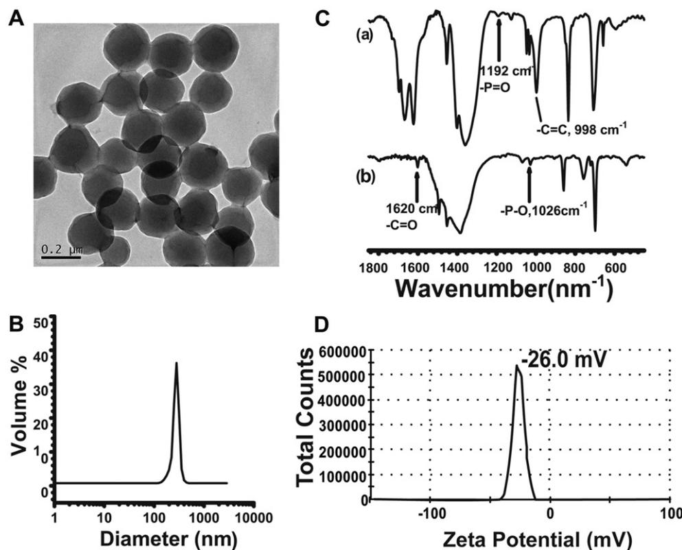
Fig. 2. (A) TEM image and (B) particle size distribution of PSt sub-micron spheres obtained from emulsion polymerization with AEOPS as emulsifier with the concentration of 1.22 g/L (i.e.  $[\text{AEOPS}] = 1.22\text{ g/L}$ ); Z-average size = 247 nm, polydispersity index = 0.042; (C) IR spectra of (a) AEOPS and (b) functional PSt sub-micron spheres; and (D) The zeta potential distribution curve for PSt sub-micron spheres ( $[\text{AEOPS}] = 1.22\text{ g/L}$ ).
