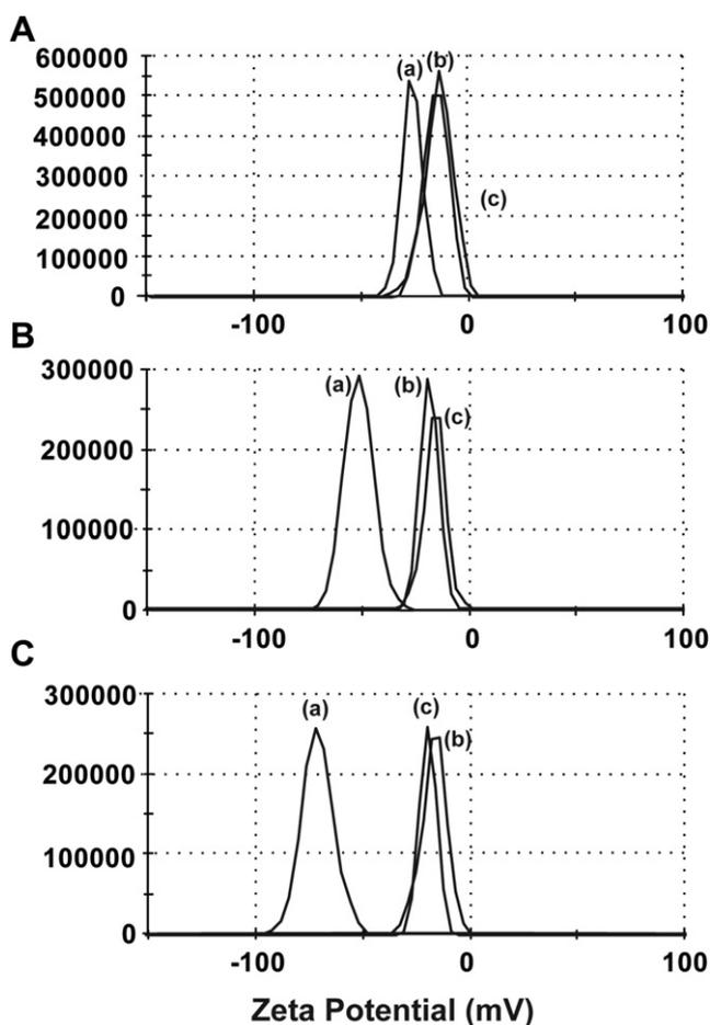
**Fig. 5.** The zeta potential distribution curves for the original PSt sub-micron spheres :  $-26.0$  mV (A, trace a),  $-51.3$  mV (B, trace a), and  $-70.7$  mV (C, trace a); PSt sub-micron sphere– $\text{Cd}^{2+}$  complex :  $-16.2$  mV (A, trace b),  $-16.5$  mV (B, trace b), and  $-19.2$  mV (C, trace b); and PSt sub-micron sphere– $\text{Pb}^{2+}$  complex :  $-16.8$  mV (A, trace c),  $-16.6$  mV (B, trace c), and  $-19.5$  mV (C, trace c).
