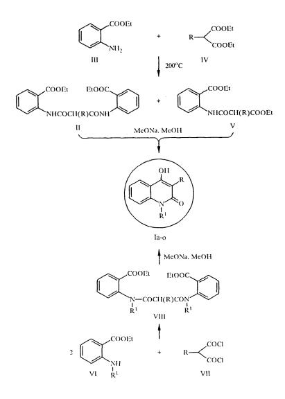
$\begin{array}{l} 1 \ R^{1} = 11; \ a \ R = C11_{3}; \ b \ R = C_{2}11_{5}; \ u \ R = CH_{2}CH=CH_{2}; \ d \ R = C_{3}11_{7}; \ e \ R = i-C_{3}11_{7}; \ f \ R = C_{4}11_{9}; \\ g \ R = C_{5}11_{11}; \ h \ R = C_{6}11_{13}; \ i \ R = C_{7}11_{15}; \ j \ R = C_{8}11_{7}; \ k \ R = C_{9}11_{19}; \ l \ R = C_{10}H_{21}; \ m \ R = C_{12}H_{25}; \\ n \ R = C1_{2}C_{6}H_{5}, \ R^{1} = C11_{3}; \ o \ R = C_{4}11_{9} \end{aligned}$
