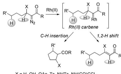
Scheme 1. Rh<sup>II</sup> carbene 1,5-C–H insertion versus 1,2-H shift.
