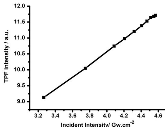
Fig. 3. The dependence of the up-converted fluorescence intensity for **1b** in H<sub>2</sub>O on the incident intensity.
