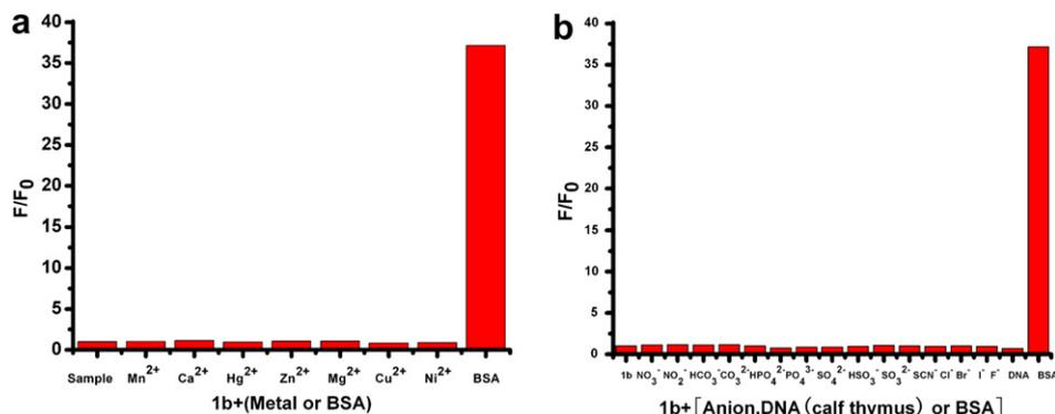
**Fig. 9.** Ratio of fluorescence intensity ( $F/F_0$  at 501 nm) of  $10 \mu\text{mol L}^{-1}$  dye **1b** in the presence of different metal ions ( $50 \mu\text{mol L}^{-1}$ ) (a), anion ( $50 \mu\text{mol L}^{-1}$ ) and DNA ( $100 \mu\text{mol L}^{-1}$ ) (b), in PBS buffer solutions (pH 7.0) at room temperature. Excitation: 380 nm.
