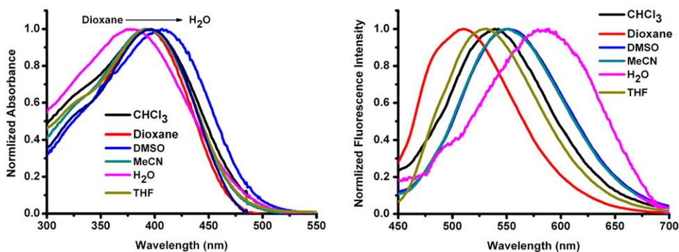
Fig. 4. One-photon absorption (left), emission spectra (right) of **1b** ( $10 \mu\text{mol L}^{-1}$ ).
