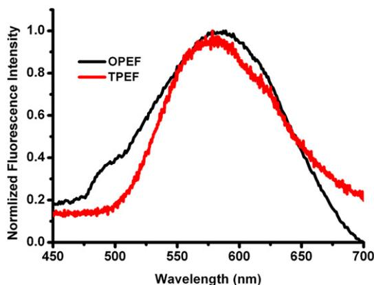
Fig. 5. OPEF and TPEF spectra of **1b** in water. OP Excitation: 380 nm, TP Excitation: 820 nm.
