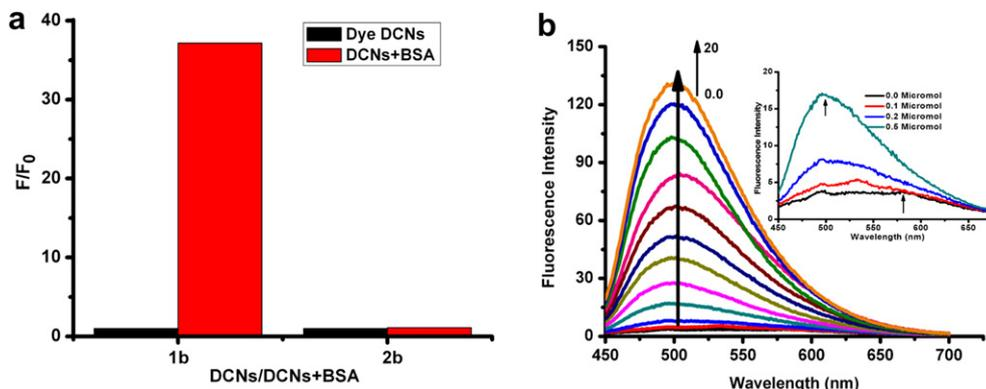
Fig. 7. a. Ratio of fluorescence intensity (**1b**:  $F/F_0$  at 501 nm, **2b**:  $F/F_0$  at 467 nm) of  $10 \mu\text{mol L}^{-1}$  dye DCNs in the presence of BSA ( $2 \mu\text{mol L}^{-1}$ ). b. Fluorescence spectra of  $10 \mu\text{mol L}^{-1}$  dye **1b** binding with BSA in PBS buffer solutions (pH 7.0) at room temperature. Excitation: 380 nm.
