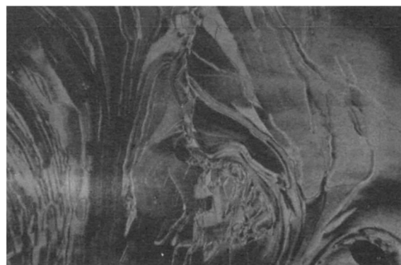
Figure 1. Photomicrograph of bis( N -hexyloxy, 4-decyloxybenzoyloxy)salicylaldiminato)nickel(II) in its nematic phase at 155^{\circ}\text{C} viewed between crossed polars.
