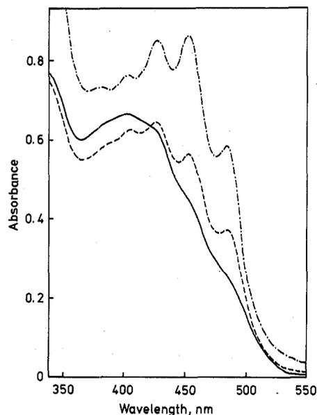
**Figure 4.** Oxidation of the product produced by anaerobic reaction of HA with acetic anhydride and pyridine. HA was reacted with pyridine and acetic anhydride under anaerobic conditions (—) and air (---) or DDQ (- · -) was added to the anaerobic mixture.
