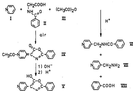
**Figure 2.** The hydrolytic cleavage of APPO formed by the reaction of HA with acetic anhydride and pyridine.
