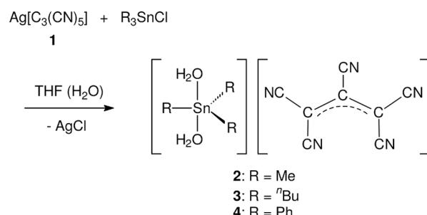
**Scheme 1.** Synthesis of the triorganotin(IV) pentacyanopropenides **2–4**.
