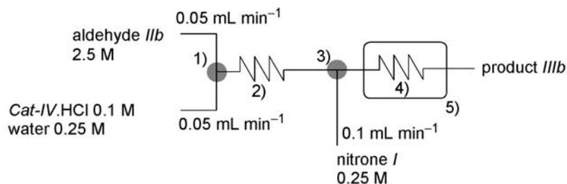
**Fig. 5.** Experimental set-up for reactions in flow microreactor: 1 – T-mixer (Teflon); 2 – residence time unit 0.5 mL (Teflon tubing); 3 – LTF MS mixer (glass); 4 – residence time unit 24 mL (Teflon tubing); 5 – heating bath.
