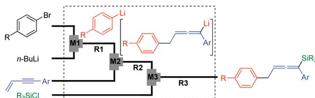
Carbolithiation of conjugated enynes with aryllithiums generated by Br–Li exchange reaction followed by reaction of the allenyllithium compounds with chlorosilanes was carried out in a microflow system to obtain various allenylsilanes in good yields.
