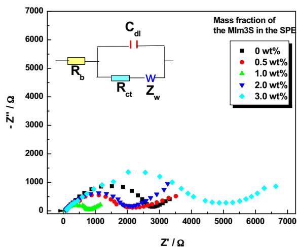
**Fig. 2.** Nyquist curves of the solid polymer electrolytes containing various amounts of the 1-(1-methyl-3-imidazolium)propane-3-sulfonate at room temperature. (Insert: equivalent circuit of the Li/SPE/Li cell).
