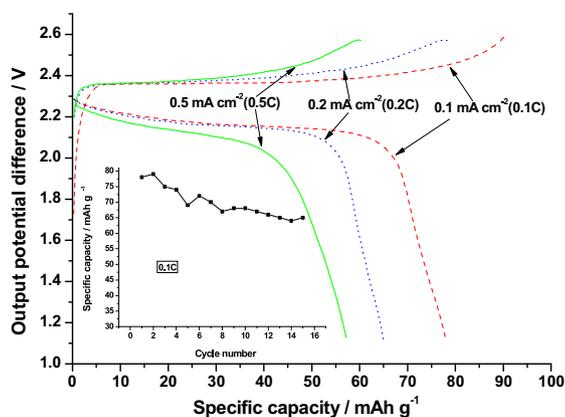
Fig. 7. Galvanostatic curves of the  $\text{Li}_4\text{Ti}_5\text{O}_{12}/\text{SPE}/\text{LiCoO}_2$  cell at various current densities of 0.1, 0.2 and  $0.5 \text{ mA cm}^{-2}$  at room temperature. The used solid polymer electrolyte contains 1 wt% of the 1-(1-methyl-3-imidazolium)propane-3-sulfonate. (Insert: cycle performance of the test cell at 0.1C).
