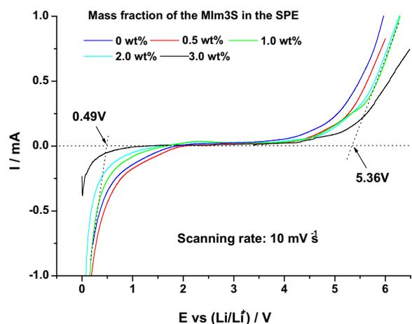
**Fig. 6.** Linear sweep voltammograms of the solid polymer electrolytes incorporated with various amounts of the 1-(1-methyl-3-imidazolium)propane-3-sulfonate at a sweep rate of  $10 \text{ mV s}^{-1}$  at room temperature. (Working electrode: stainless steel; reference and counter electrodes: lithium).
