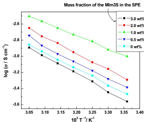
**Fig. 5.**  $\log \sigma - T^{-1}$  curves of the solid polymer electrolytes incorporated with various amounts of the 1-(1-methyl-3-imidazolium)propane-3-sulfonate in the range of  $25\text{--}55^\circ\text{C}$ .
