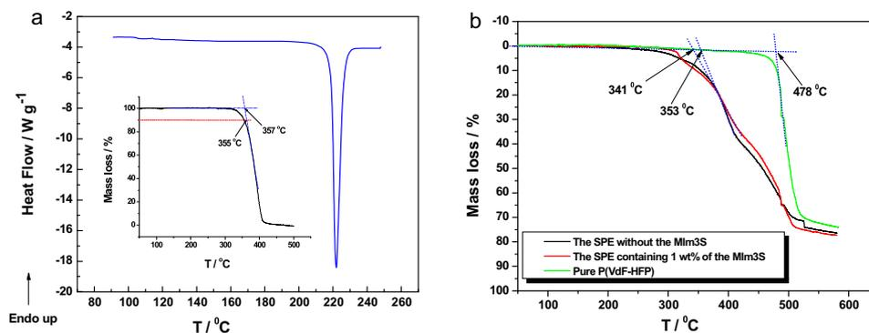
**Fig. 1.** (a) Differential scanning calorimetry and thermogravimetric curves of the 1-(1-methyl-3-imidazolium)propane-3-sulfonate measured in a  $N_2$  atmosphere at a scan rate  $10^\circ\text{C min}^{-1}$ . (Insert: thermogravimetric curve); (b) Thermogravimetric curves of the solid polymer electrolytes incorporated without and with 1.0 wt% of the 1-(1-methyl-3-imidazolium)propane-3-sulfonate.
