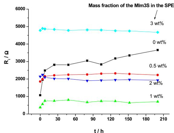
**Fig. 3.** Interfacial resistances of the solid polymer electrolytes incorporated with various amounts of the 1-(1-methyl-3-imidazolium)propane-3-sulfonate at room temperature after different storage time.
