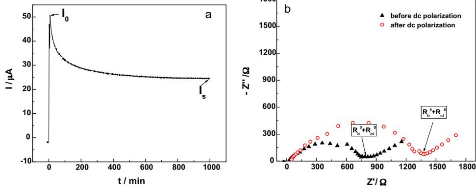
**Fig. 4.** Chronoamperometry profile (a) and Nyquist plots (b) of the solid polymer electrolytes containing 1.0 wt% of the 1-(1-methyl-3-imidazolium)propane-3-sulfonate at room temperature.
