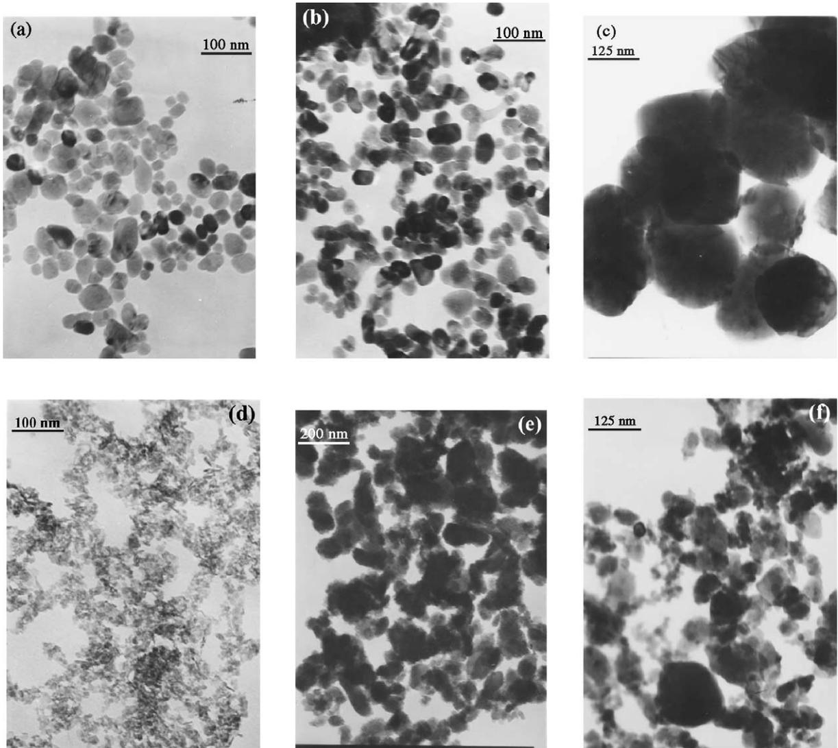
Fig. 3. TEM images of typical samples of nanocrystalline tungstates: (a)  $\text{CaWO}_4$ , (b)  $\text{SrWO}_4$ , (c)  $\text{BaWO}_4$ , (d)  $\text{CdWO}_4$ , (e)  $\text{ZnWO}_4$ , (f)  $\text{PbWO}_4$ .
