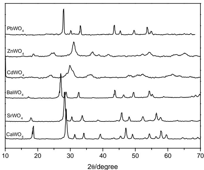
Fig. 2. XRD patterns of as-obtained nanocrystalline tungstates:  $\text{CaWO}_4$ ,  $\text{SrWO}_4$ ,  $\text{BaWO}_4$ ,  $\text{CdWO}_4$ ,  $\text{ZnWO}_4$ , and  $\text{PbWO}_4$ .
