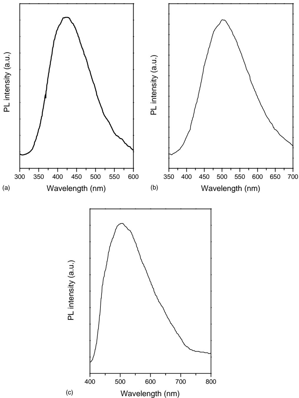
Fig. 4. Photoluminescence (PL) spectrum of as-prepared nanocrystalline tungstates: (a)  $\text{CaWO}_4$ , (b)  $\text{CdWO}_4$ , (c)  $\text{PbWO}_4$ .
