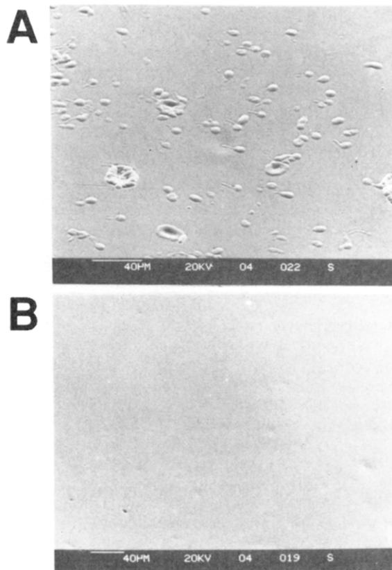
**Figure 3.** (A) SEM of surface of unphotolyzed DHA electrode in Figure 2, after 78 days of aqueous storage. (B) SEM of surface of photolyzed DHA electrode in Figure 4, after 78 days of aqueous storage. Electrode B had not failed at time of removal from solution.
