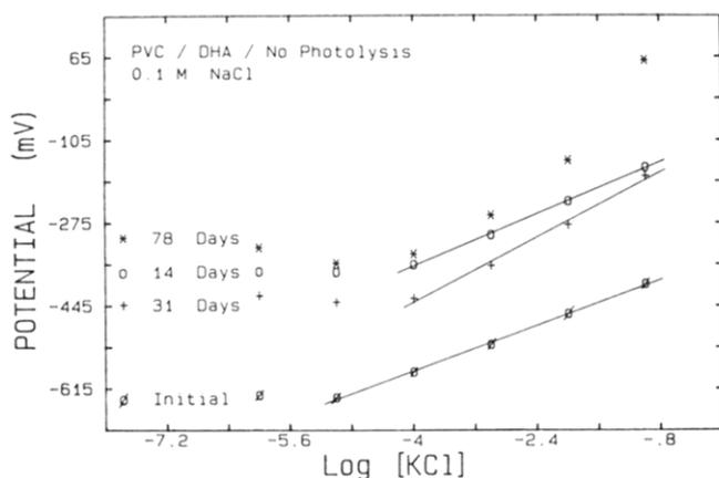
**Figure 2.** Plot of potential versus log [KCl] in 0.1 M NaCl for DHA and 0.25% AIBN plasticized membrane coated on an n-Si electrode during 78 days of storage in  $10^{-5}$  M KCl, 0.1 M NaCl.
