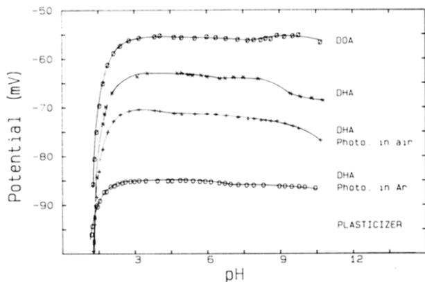
**Figure 1.** pH response of ion selective electrode configured membranes plasticized with ( $\phi$ ) DOA, (\*) DHA and 2.5% AIBN; (+) 30 min, air-photolyzed DHA and 2.5% AIBN, and (O) 30-min photolysis under Ar, DHA, and 2.5% AIBN. Measured in 1 mM KCl with 10 mM phosphate as buffer. pH was adjusted with 1 mM KCl, 0.1 M HCl and 1 mM KCl, 0.1 M NaOH.
