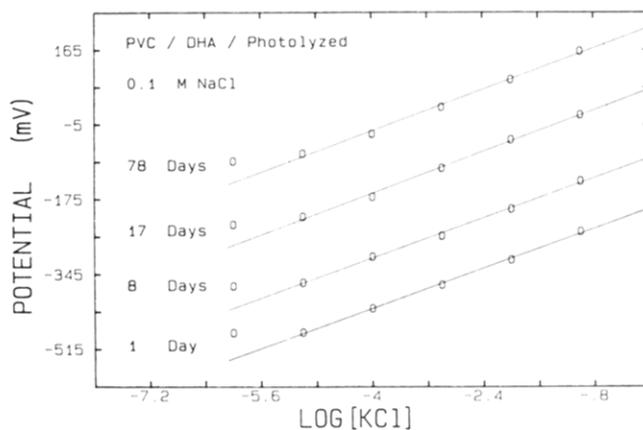
**Figure 4.** Plot of potential versus log [KCl] in 0.1 M NaCl for DHA and 0.25% AIBN plasticized membrane coated on n-Si electrode after 30 min of photolysis in air, during 78 days of storage in  $10^{-5}$  M KCl, 0.1 M NaCl.
