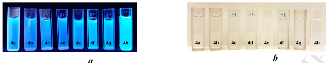
Fig. 3 (a) Photographs of the solutions of 4a-h under irradiation with hand-held UV lamp at emission wavelength of 380 nm. (b) Photographs of the same solutions taken under daylight.
