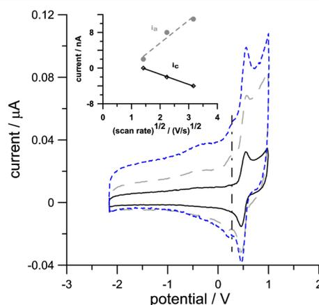
**Figure 5.** Cyclic voltammetric curves of compound **7** in 0.05 M TBAHFP/DMSO solution;  $T = 298$  K;  $\nu = 0.2$  (solid line), 0.5 (long dashed line), 10 V s<sup>-1</sup> (short dashed line); working electrode Pt disk ( $d = 125$  μm). The inset gives the scan rate dependence of the shoulder indicated by the dash-dotted line on the CV curves. Potentials are referenced to the SCE.
