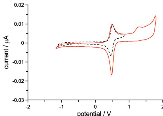
**Figure 1.** Cyclic voltammetric curves of compound **5** (0.8 mM) in 0.05 M TBAHFP/DCM solution, recorded with two different scan reversal potentials:  $T = 298 \text{ K}$ ;  $\nu = 0.5 \text{ V s}^{-1}$ ; working electrode Pt disk ( $d = 125 \mu\text{m}$ ). Potentials are referenced to the SCE.
