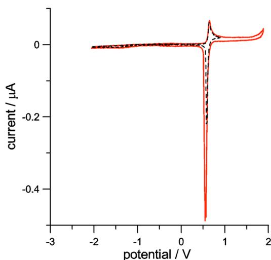
**Figure 6.** Cyclic voltammetric curves of compound **14** (0.8 mM) in 0.05 M TBAHFP/DCM solution:  $T = 298$  K;  $\nu = 0.5$  V s<sup>-1</sup>, recorded with two different scan reversal potentials; working electrode Pt disk ( $d = 125$  μm). Potentials are referenced to the SCE.
