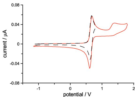
**Figure 7.** Cyclic voltammetric curves of compound **18** (0.8 mM) in 0.05 M TBAHFP/DCM solution:  $T = 298$  K;  $\nu = 0.5$  V s<sup>-1</sup>, recorded with two different scan reversal potentials; working electrode Pt disk ( $d = 125$  μm). Potentials are referenced to SCE.
