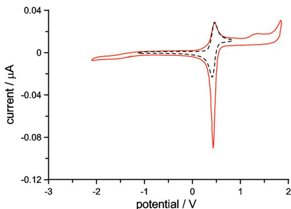
**Figure 2.** Cyclic voltammetric curves of compound **7** (0.8 mM) in 0.05 M TBAHFP/DCM solution:  $T = 298$  K;  $\nu = 0.5$  V s<sup>-1</sup>, recorded with two different scan reversal potentials; working electrode Pt disk ( $d = 125$  μm). Potentials are referenced to the SCE.
