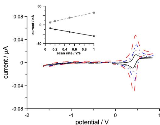
**Figure 3.** Cyclic voltammetric curves of compound **7** (0.8 mM) in 0.05 M TBAHFP/DCM solution:  $T = 298$  K;  $\nu = 0.1$  (solid line), 0.2 (short dashed line), 0.5 (dash-dotted line), 1 V s<sup>-1</sup> (long dashed line); working electrode Pt disk ( $d = 125$  μm). The inset gives peak currents as a function of scan rate. Potentials are referenced to the SCE.
