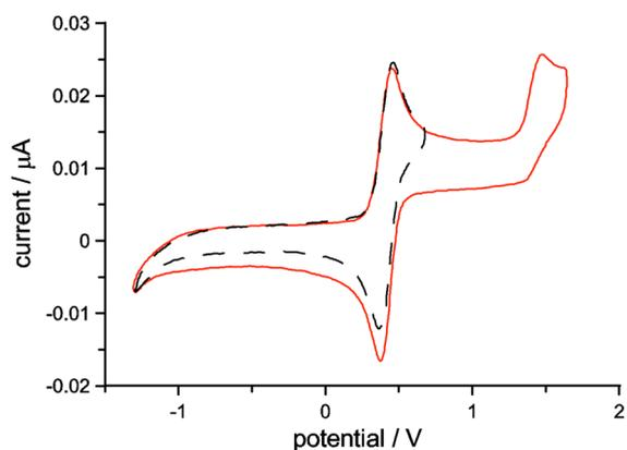
**Figure 4.** Cyclic voltammetric curves of compound **12** (0.8 mM) in 0.05 M TBAHFP/DCM solution:  $T = 298$  K;  $\nu = 0.5$  V s<sup>-1</sup>, recorded with two different scan reversal potentials; working electrode Pt disk ( $d = 125$  μm). Potentials are referenced to the SCE.
