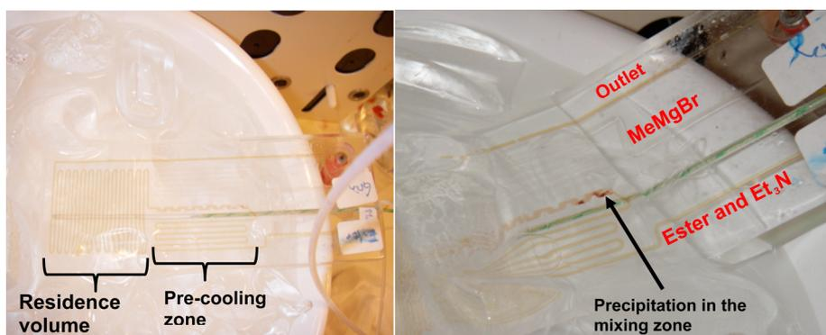
**Figure 3.** Picture of the Sigma-Aldrich glass chip reactor used for the mixing of MeMgBr and solution of ester **1**/Et<sub>3</sub>N.
