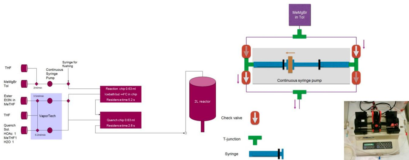
Figure 2. Schematic setup for the continuous processing in the Aldrich chip reactor and continuous syringe pump.
