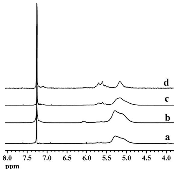
**Fig. 3.** <sup>1</sup>H NMR spectra of typical PENB samples from (a) run 2, (b) run 4, (c) run 9 and (d) run 10 in Table 3 (recorded in CDCl<sub>3</sub> at room temperature).
