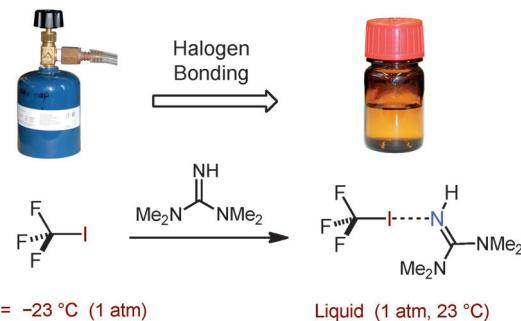
**Figure 1.** Formation of liquid TMG- $\text{CF}_3\text{I}$  adduct via halogen bonding between  $\text{CF}_3\text{I}$  and tetramethylguanidine (TMG).
