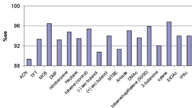
**Figure 1.** Percent ee as a function of solvent. Conditions: 0.5 mol % catalyst loading and 90 psig H<sub>2</sub>. All solvents gave >85% conversion.
