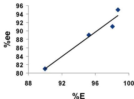
**Figure 2.** Reaction % ee plotted as a function of % E isomer in **6** (0.5 mol % catalyst loading and 90 psig H<sub>2</sub>).
