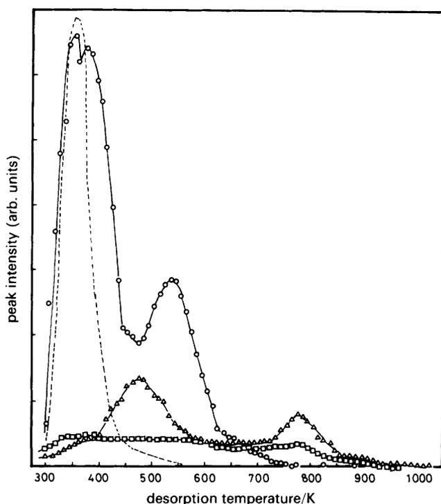
Fig. 10 TPD spectra of gases desorbed from Yb/K-Y.  $\Delta$ ,  $H_2$ ;  $\circ$ ,  $NH_3$ ;  $\square$ ,  $N_2$ . Yb (6.6 wt.%) / K-Y heated under vacuum at 303 K for 1 h after impregnation. (---) see Fig. 9
