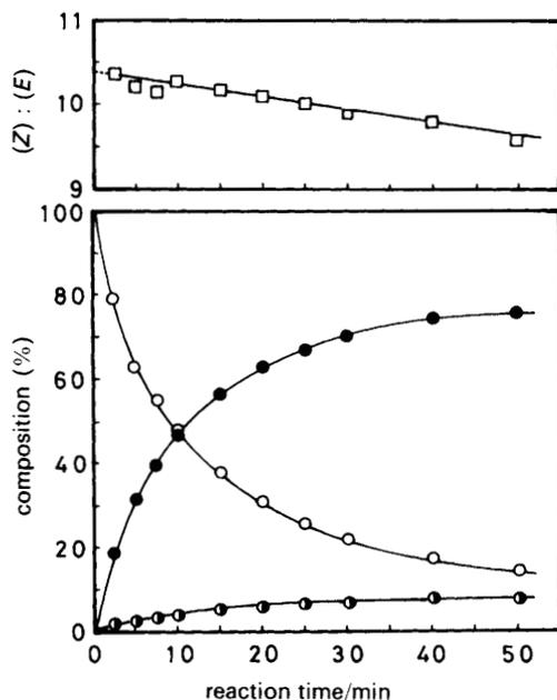
**Fig. 1** Composition change in the reaction gas with reaction time. 0.027 g of Eu supported on 0.5 g of K-Y zeolite. Catalyst heated under vacuum at 473 K for 1 h after contacting Eu solution of liquid ammonia with K-Y zeolite. Reaction temperature 273 K, pressure of but-1-ene 20.5 kPa. ○, but-1-ene; ●, (Z)-but-2-ene; ●, (E)-but-2-ene; □, (Z):(E) ratio
