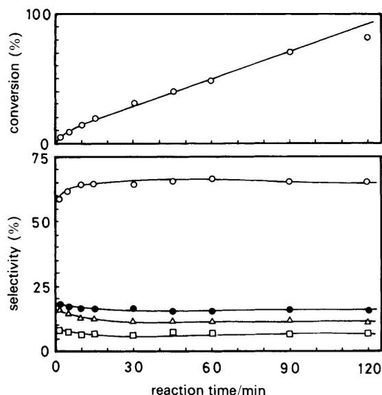
Fig. 5 Change in buta-1,3-diene conversion and selectivity to reaction products with reaction time. 0.013 g of Yb supported on 0.20 g of K-Y zeolite. Catalyst heated under vacuum at 873 K for 1 h after impregnation. Reaction temperature 323 K, hydrogen 26.6 kPa, buta-1,3-diene 13.3 kPa. ○, But-1-ene; △, (Z)-but-1-ene; ●, (E)-but-2-ene; □, butane
