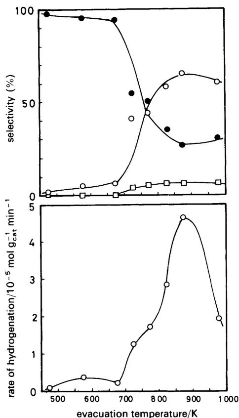
Fig. 7 Influence of evacuation temperature on the catalytic activity of Yb (6.6 wt.%) on K-Y. Reaction temperature 323 K, hydrogen 26.6 kPa, buta-1,3-diene 13.3 kPa.  $\circ$ , But-1-ene;  $\bullet$ , but-2-enes;  $\square$ , butane
