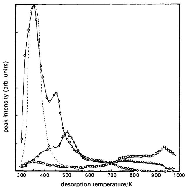
Fig. 9 TPD spectra of gases desorbed from Eu/K-Y.  $\Delta$ ,  $\text{H}_2$ ;  $\circ$ ,  $\text{NH}_3$ ;  $\square$ ,  $\text{N}_2$ . Eu (5.5 wt.%) on K-Y heated under vacuum at 323 K for 1 h after impregnation. (---)  $\text{NH}_3$  desorbed from K-Y heated under vacuum at 323 K, after contacting K-Y with liquid ammonia
