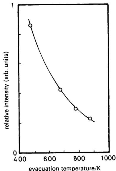
Fig. 8 Relative intensity of band emission for  $\text{Eu}^{2+}$  vs. evacuation temperature. Eu (5.5 wt.%) supported on K-Y zeolite. Eu/K-Y catalyst heated under vacuum at the prescribed temperature
