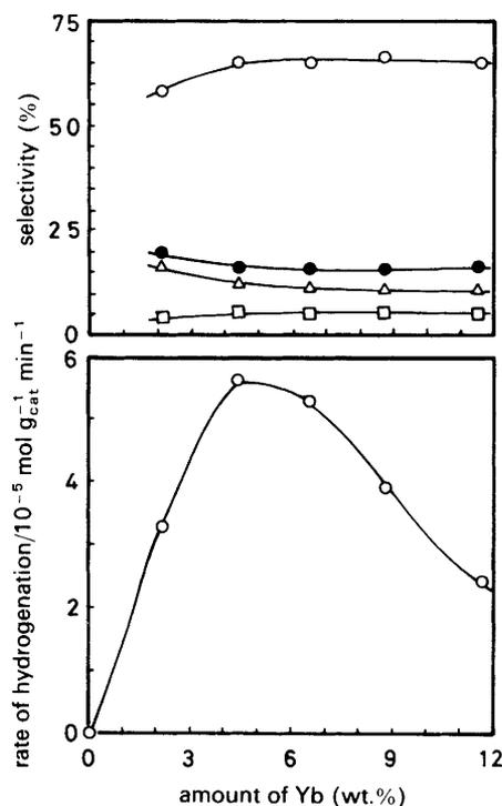
Fig. 6 Dependence of the catalytic activity for hydrogenation of buta-1,3-diene on the amount of Yb supported on K-Y zeolite. Reaction conditions: see Fig. 5
