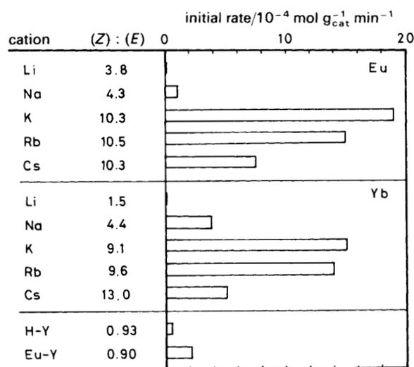
**Fig. 2** Catalytic activity of Eu or Yb supported on alkali-metal cation-exchanged Y-zeolite. Degree of cation exchange: Li (67%), Na (100%), K (99%), Rb (47%) and Cs (39%). Reaction conditions: see Fig. 1
