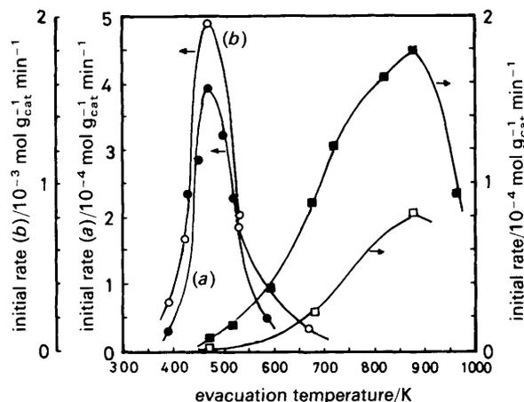
Fig. 4 Influence of evacuation temperature on the catalytic activity for isomerization of but-1-ene and hydrogenation of ethene. Isomerization of but-1-ene: ●, Yb (6.6 wt.%) / Na-Y; ○, Eu (5.5 wt.%) / K-Y. Reaction temperature 273 K, but-1-ene: 20.5 kPa. Hydrogenation of ethene: ■, Yb (6.6 wt.%) supported on K-Y zeolite; □, Eu (5.5 wt.%) / K-Y. Reaction temperature 273 K, hydrogen 26.6 kPa, Ethene 13.3 kPa
