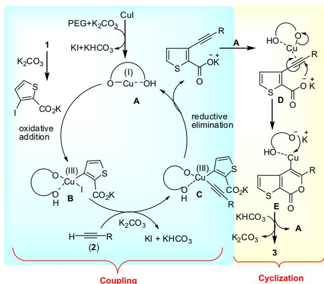
**Scheme 2.** Proposed mechanism for the Cu-mediated coupling-cyclization of **1** with **2** in PEG under ultrasound.
