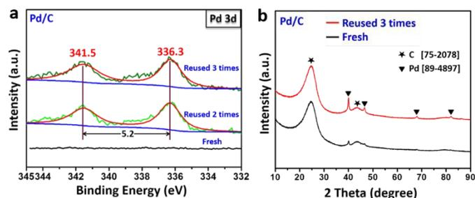
Fig. 1 XPS spectra of fresh and reused Pd/C (a). XRD patterns of fresh and reused Pd/C (b).
