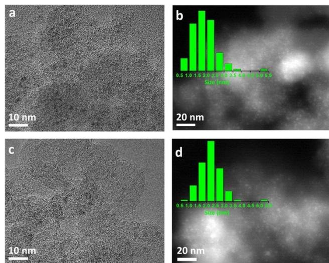
Fig. 2 TEM (a, c) and HAADF-STEM (b, d) images of the fresh Pd/C (a, b), reused Pd/C (c, d).
