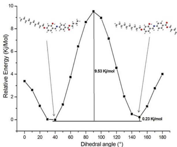
**Figure 8.** Potential energy vs dihedral angle ( $-C_{17}-C_{16}-N_{12}-C_{10}-$ ) curve of butyl 4-(4'-(decyloxy)-2-hydroxybenzylideneamino)benzoate.
