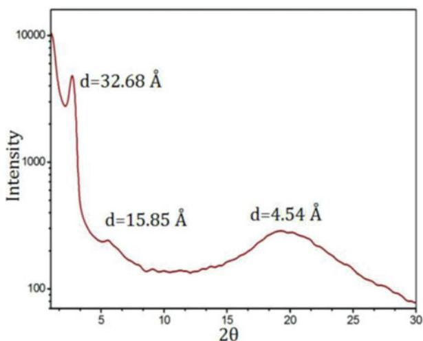
**Figure 6.** XRD diffractogram at 60°C during the cooling cycle of butyl 4-(4'-(dodecyloxy)-2-hydroxybenzylideneamino)benzoate.
