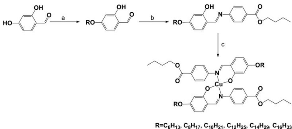
**Scheme 1.** Reactions and reagents: (a) RBr (1.0 equiv.), potassium hydrogen carbonate (1.1 equiv.), refluxing in 2-butanone, 30 h (b) butyl 4-aminobenzoate (1.0 equiv.), acetic acid (4–5 drops), refluxing in ethanol, 4 h (c)  $\text{Cu}(\text{OAc})_2 \cdot \text{H}_2\text{O}$  (0.5 equiv.), stirring, 4 h.
