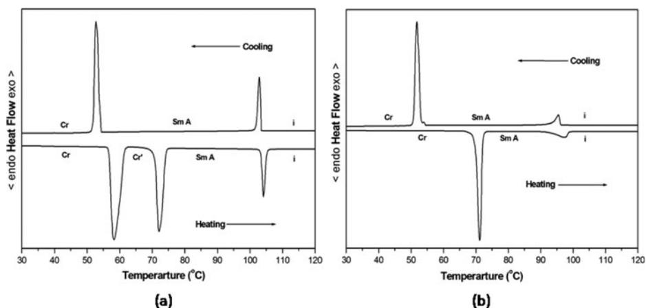
**Figure 1.** DSC thermogram of (a) butyl 4-(4'-(octyloxy)-2-hydroxybenzylideneamino)benzoate (b) butyl 4-(4'-(hexadecyloxy)-2-hydroxybenzylideneamino)benzoate.
