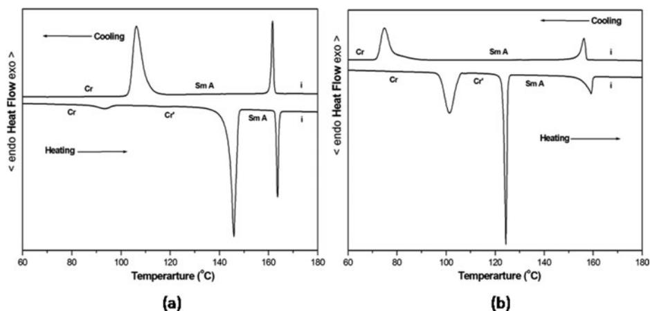
**Figure 4.** DSC thermogram of (a) copper(II) complex of butyl 4-(4'-(octyloxy)-2-hydroxy benzylideneamino)benzoate (b) copper(II) complex of butyl 4-(4'-(dodecyloxy)-2-hydroxy benzylideneamino)benzoate.
