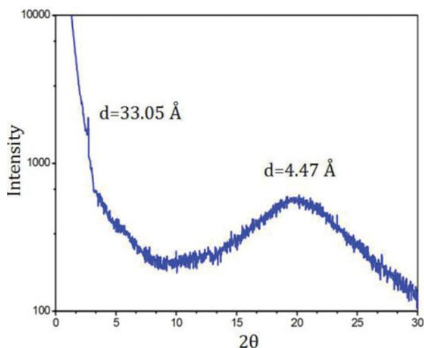
**Figure 3.** XRD diffractogram at 60°C during the cooling cycle of butyl 4-(4'-(dodecyloxy)-2-hydroxybenzylideneamino)benzoate.
