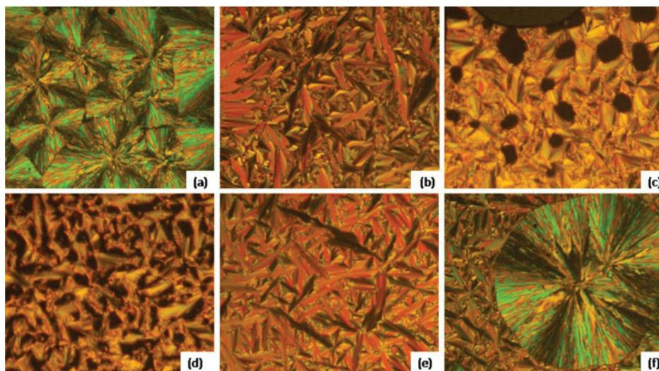
**Figure 5.** Optical textures of copper(II) complex of butyl 4-(4'-(dodecyloxy)-2-hydroxybenzylideneamino)benzoate under a polarizing optical microscopy. Heating cycle: (a) crystal phase at 112°C (b) SmA mesophase at 140°C (c) SmA mesophase to isotropic transition at 159°C. Cooling cycle: (d) Isotropic to SmA mesophase at 156°C (e) SmA mesophase at 130°C (f) SmA mesophase to crystal transition at 75°C.
