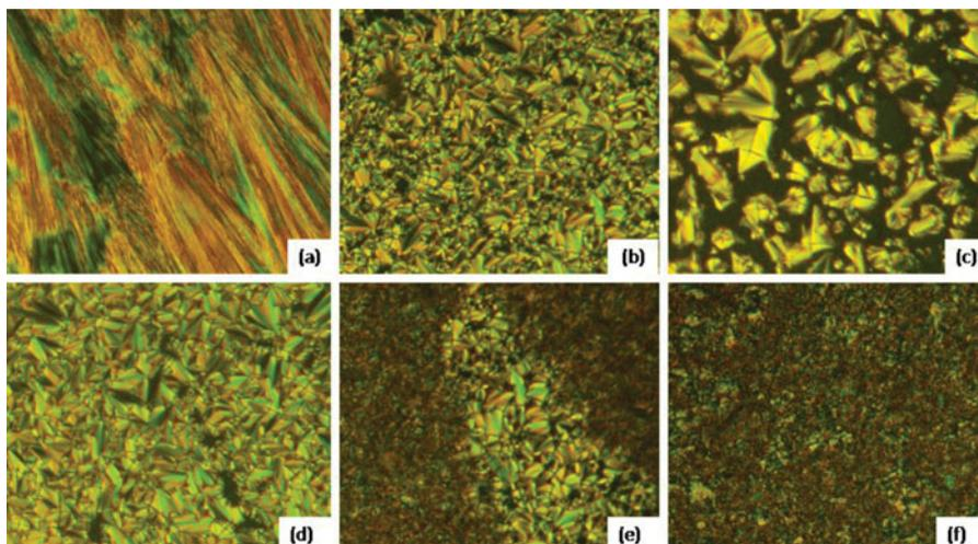
**Figure 2.** Optical textures of butyl 4-(4'-(dodecyloxy)-2-hydroxybenzylideneamino)benzoate under a polarizing optical microscopy. Heating cycle: (a) crystal phase at 60°C (b) SmA mesophase at 90°C (c) SmA mesophase to isotropic transition at 101°C. Cooling cycle: (d) SmA mesophase at 96°C (e) SmA mesophase to crystal transition at 36°C (f) Crystal phase at 35°C.
