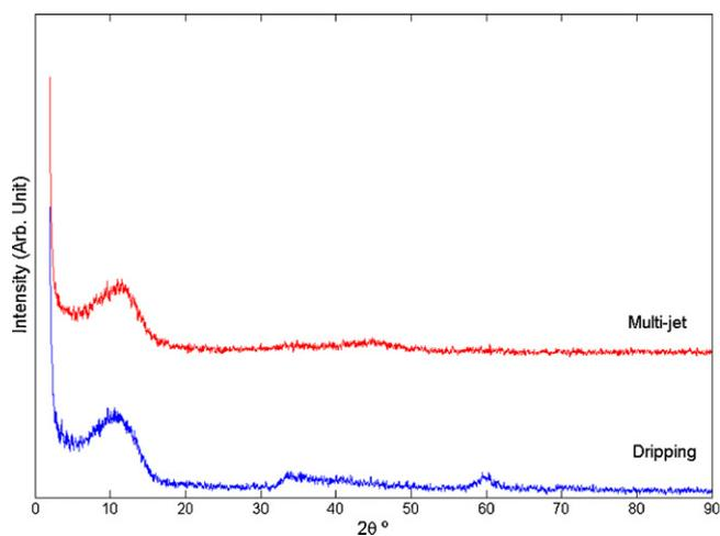
Fig. 4. XRD patterns of nickel nanoparticles synthesized in dripping and multi-jet mode.
