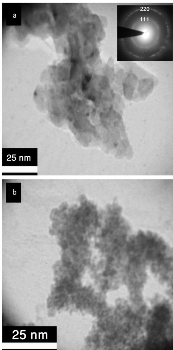
Fig. 3. TEM image of nickel nanoparticles synthesized in (a) dripping and (b) multi-jet mode and SAED pattern of particles (inset at a).
