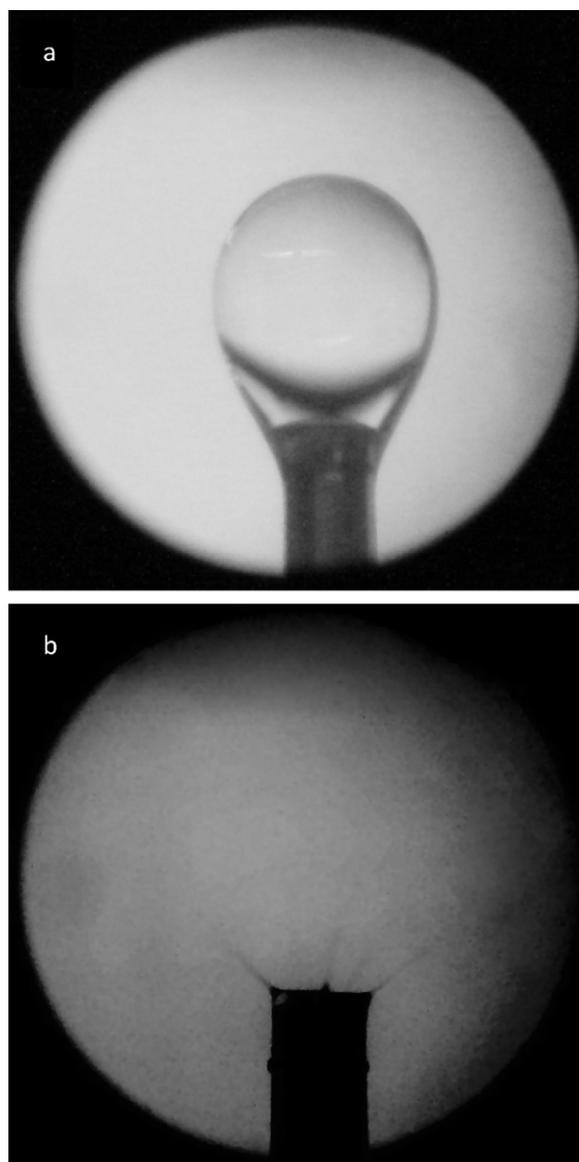
Fig. 2. Images of (a) dripping and (b) multi-jet mode.
