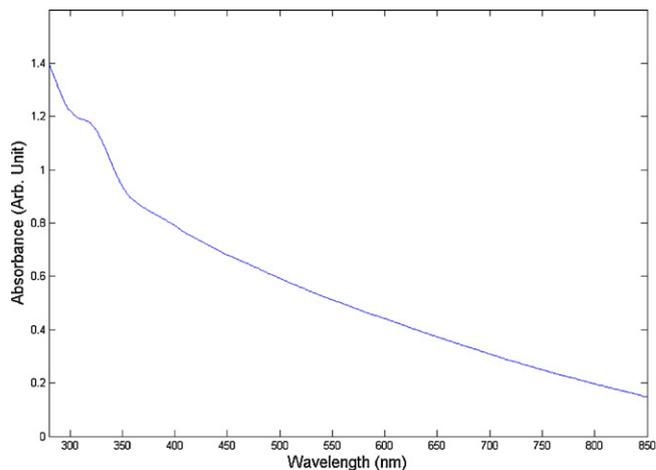
Fig. 5. UV-Visible absorption spectrum of Ni nanoparticles synthesized in multi-jet mode dispersed in methanol.
